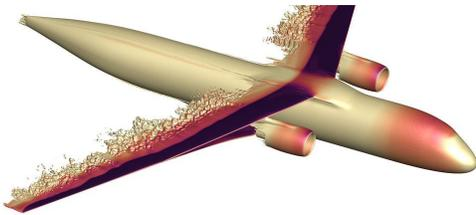
“No, it’s not hypermodern art. This image, generated by NASA’s high-performance computers, shows a Transonic Truss Braced Wing (TTBW) aircraft concept being tested in a virtual wind tunnel, showing how its wings interact with the air around them.
